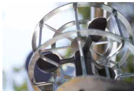
Anemometer (optional) For monitoring and warning that the maximum permissible wind speed (45km/h) has been reached.
