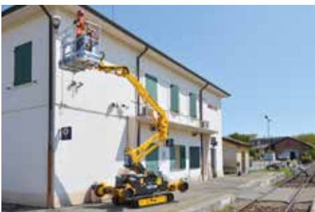
Flexibility at the top operating the machine on tracks or on ground without any stabilization even in narrow doorways.
