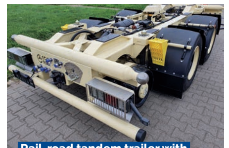
Rail-road tandem trailer with 10 or 20 foot twist lock swap body system
